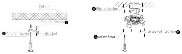
Attention: Must secure mounting plate at all connection points (junction box plus four outer points for small and medium size, or six outer points for large size) to support fixture weight appropriately. Not using all mounting points could damage the fixture and void product warranty.
