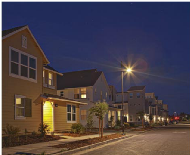
Figure 6. The City of Davis has specified a low-wattage, 2700K roadway fixture for their residential roadways.
