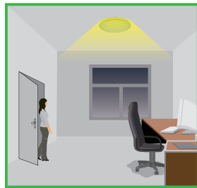
With insufficient natural light, the sensor switches on the light automatically when presence is detected.
