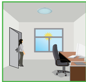
With sufficient natural light, the light does not switch on when presence is detected.
