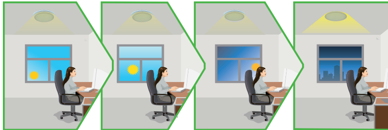
The light turns on at full or dims to maintain the lux level. The light output regulates according to the level of natural light available.
