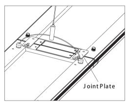
1) Joint two luminaires together by mounting the Joint plate on the both sides as shown.
