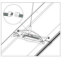
2 Remove the existing covers, then connect the quick connectors properly.
