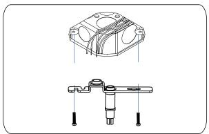
2.Attach the hanging cable and suspension cable by pushing them through the holes on the canopy, and fix the suspension cable of the attachment point Then Connect AC wires and dimming wires.
