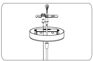
3.Put the cover against the ceiling, then screw the cap into base clockwise.
