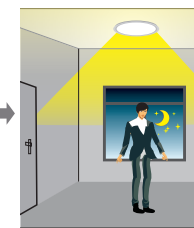
The lamp lights on 100% illumination or dims to maintain the preset illumination level against the level of ambient light.
